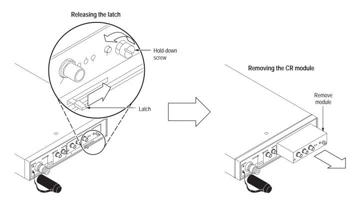
Figure 8: Releasing the module with the latch
