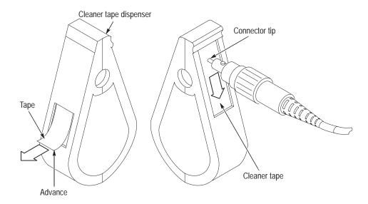
Figure 20: Cleaning an optical connector
