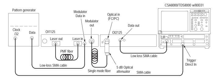
Figure 2: Functional test setup
