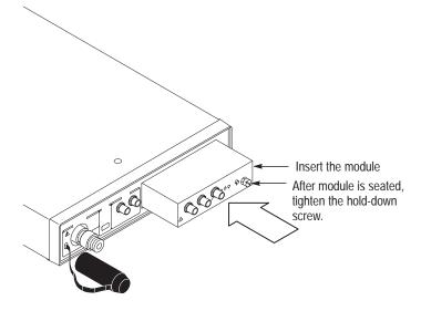
Figure 7: Installing a Clock Recovery Module
