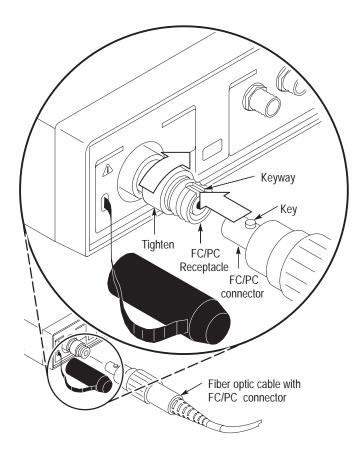
Figure 4: Connecting a fiber optic cable
