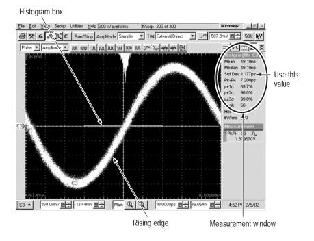
Figure 19: RMS Jitter measurement
