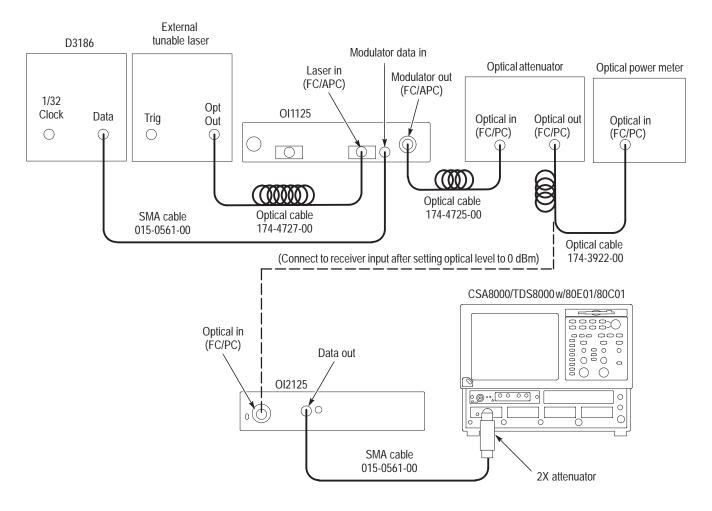
Figure 16: Setup for the eye pattern test matrix
