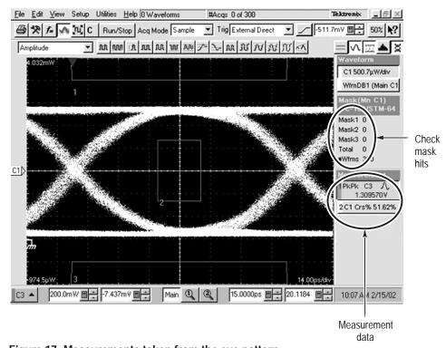
Figure 17: Measurements taken from the eye pattern
