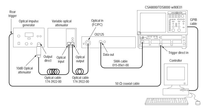
Figure 14: Setup for the bandwidth test
