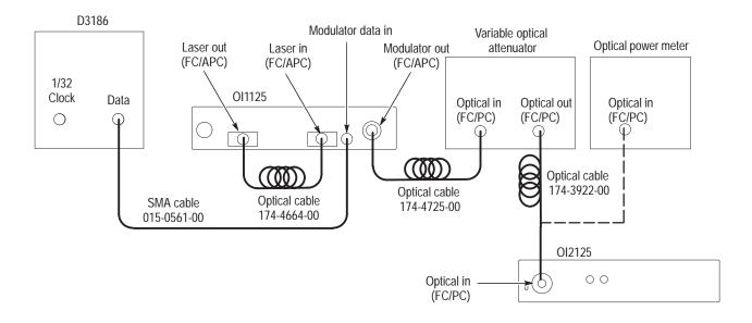
Figure 13: Setup for the LOS threshold test
