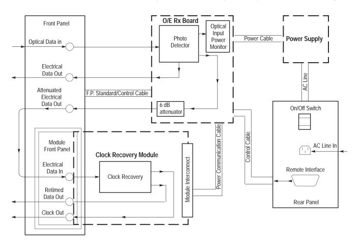
Figure 12: O/E Receiver interconnect diagram
