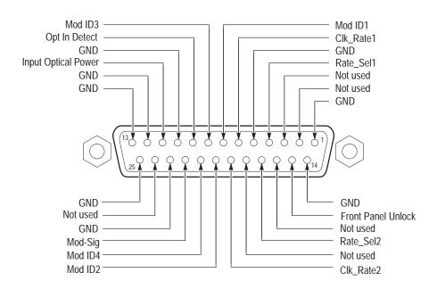
Figure 10: Rear Remote Interface connector pinout
