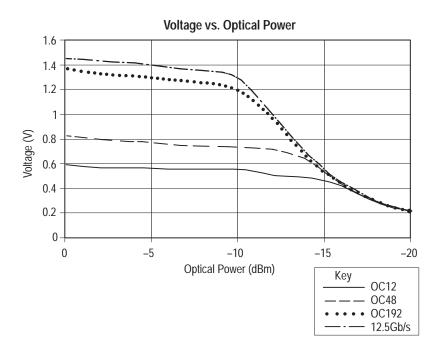
Figure 11: Ol2125 Output Voltage versus Input Optical Power
