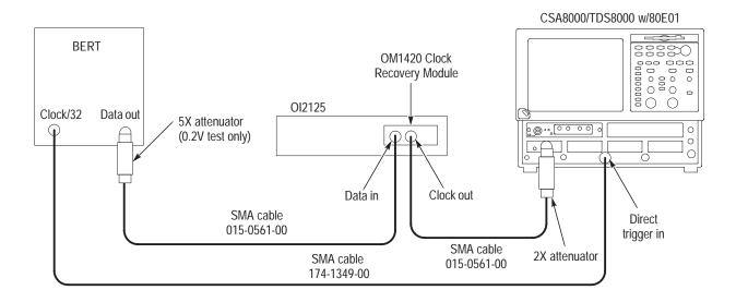
Figure 18: OM1420 Clock Recovery Module test setup
